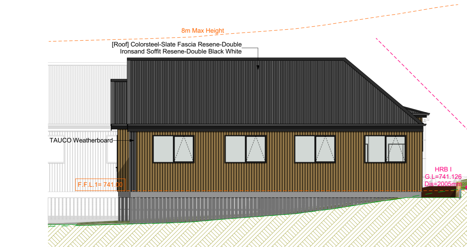
West Elevation BLOCK 1
