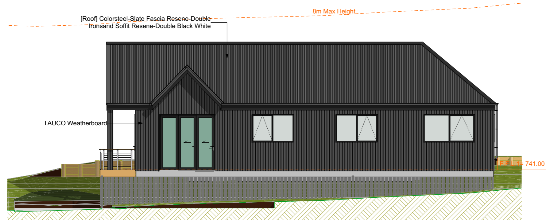
West Elevation BLOCK 2
